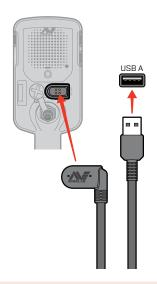
Charge your detector with a good-quality USB charger that has a minimum charging capacity of 2A @ 5V.
